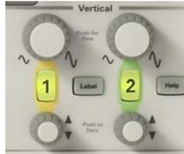
Figure 7. Position Controls for Channels 1 and 2.
