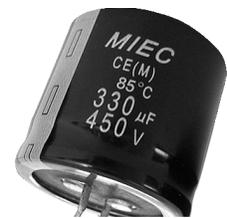
Electrolytic capacitors are polarized. When using these capacitors in a circuit they must be connected in the correct polarity. The voltage rating on an electrolytic capacitor indicates its maximum continuous operating voltage. It is important that electrolytic capacitors be used correctly. If an electrolytic capacitor is operated beyond its rated voltage or wired incorrectly (reverse polarized) it may be damaged and even explode!
