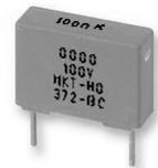
Polyester film capacitors have the capacitance value along with the unit printed on the case. Other information such as the voltage rating and the manufacturer's part or series number may also be shown. In the picture the capacitance value is 100nF (or 0.1 $\mu$ F) and the voltage rating is 100V (DC).
